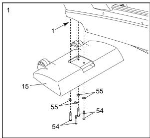
While another person lifts the rear of the Frame (1), attach the Rear Stabilizer (16) to the Frame with four M8 x 40mm Button Screws (54) and four M8 Split Washers (55).
